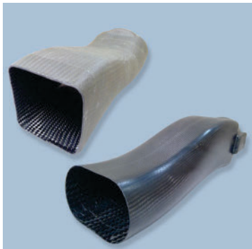
VARTM composite duct next to Smart Tool mandrel that contracts inside mold line (IML) during cure.
