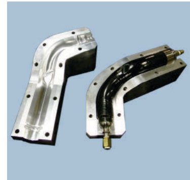
Smart Tool mandrel used to mold a composite duct shown in forming mold
