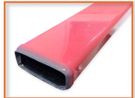
Figure 7 - Close-up of Smart Tool with FEP release film
