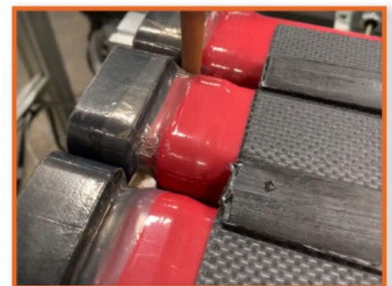
Figure 3 - Custom molded noodles fitted in-between Smart Tools to create flush surface
