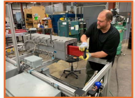
Figure 5 - Smart Tools being extracted while still elastic from the cured composite
