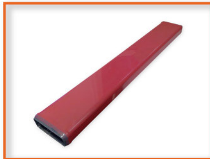
Figure 6 - Smart Tool with FEP release film
