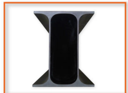
Figure 9 - Completed composite I-Beam end view
