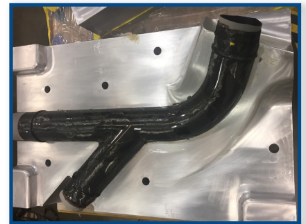
Smart Tool inside cured composite vent tube
