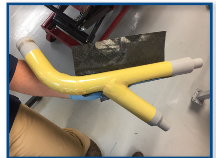
Coated Smart Tool with non-permeable liner
