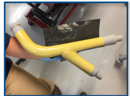
Coated Smart Tool with non-permeable liner
