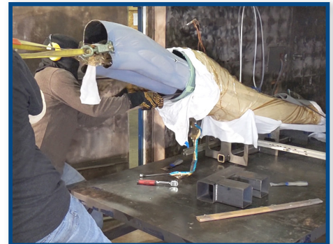
Elastic Smart Tool being extracted from cured composite part
