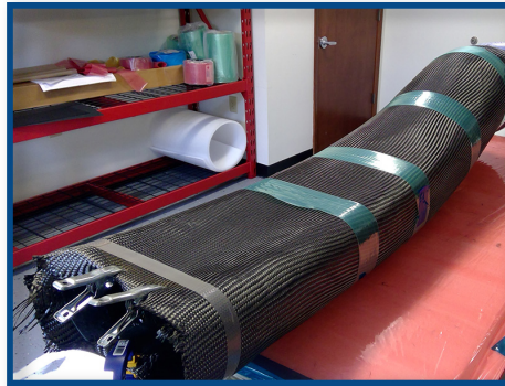
Dry carbon fiber braided sleeving secured to smart tool
