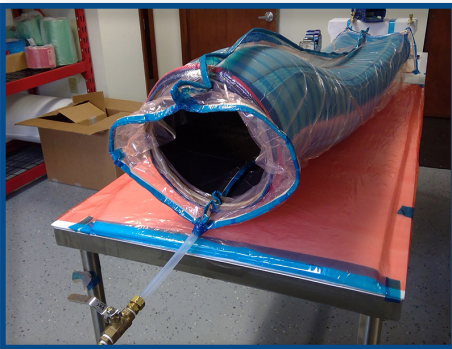
Vacuum bags attached both on the inside and outside of Smart Tool
