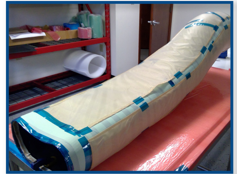
Mandrel wrapped with release ply and flow media strip
