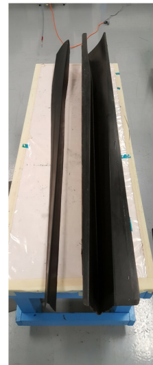
Demolded Smart Tool Caul & composite part
