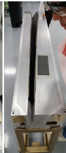
How Smart Tool Caul fits into female mold
